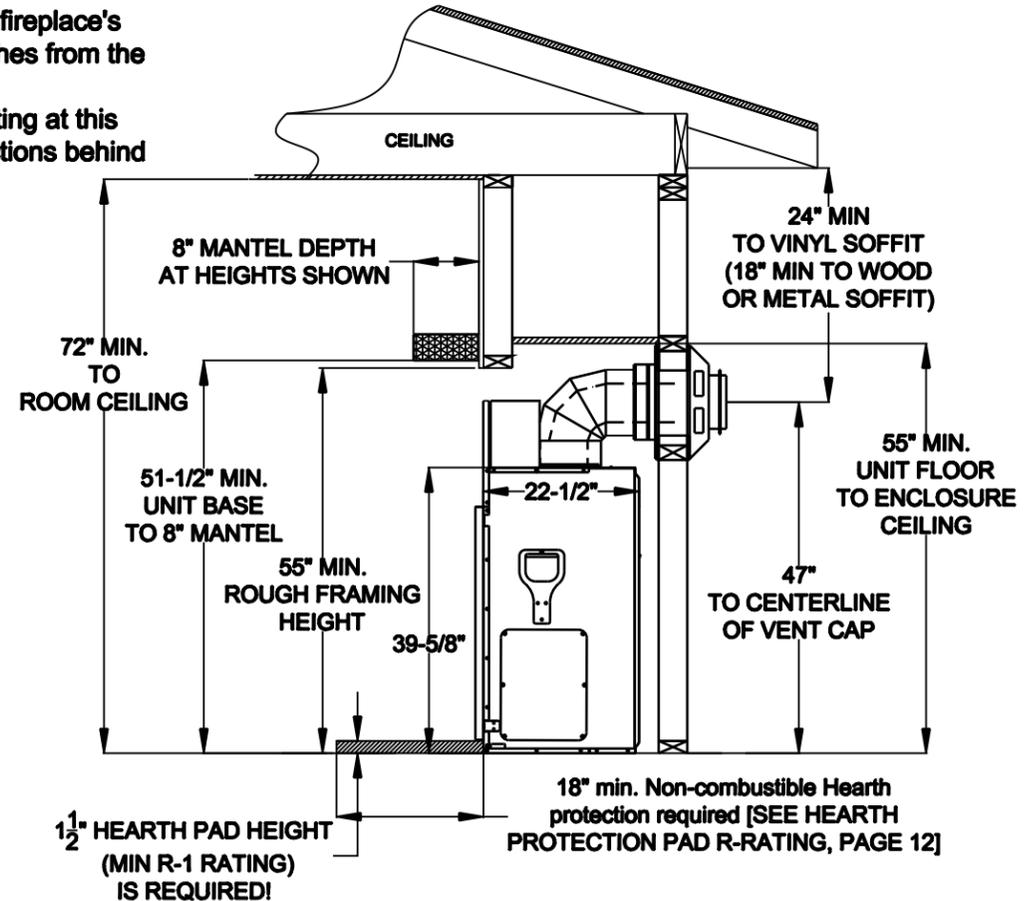
**NOTE:** For every 1" this fireplace is raised off the floor, the non-combustible hearth protection pad may be reduced by 2". If this fireplace is raised off the floor more than 6", No hearth protection pad is required.
