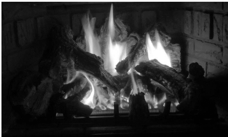
Figure 6-2 Burner Flame Heights: This image provides a visual reference for the burner flames burning at maximum height after the burners have been operating for 30 minutes or longer. A normal rear flame will be 1 to 2 inches above the rear log top edge. This, however, is dependent on the gas type, air shutter opening setting and vent system configuration. Actual flame heights can be slightly higher or lower when compared to this reference image.
