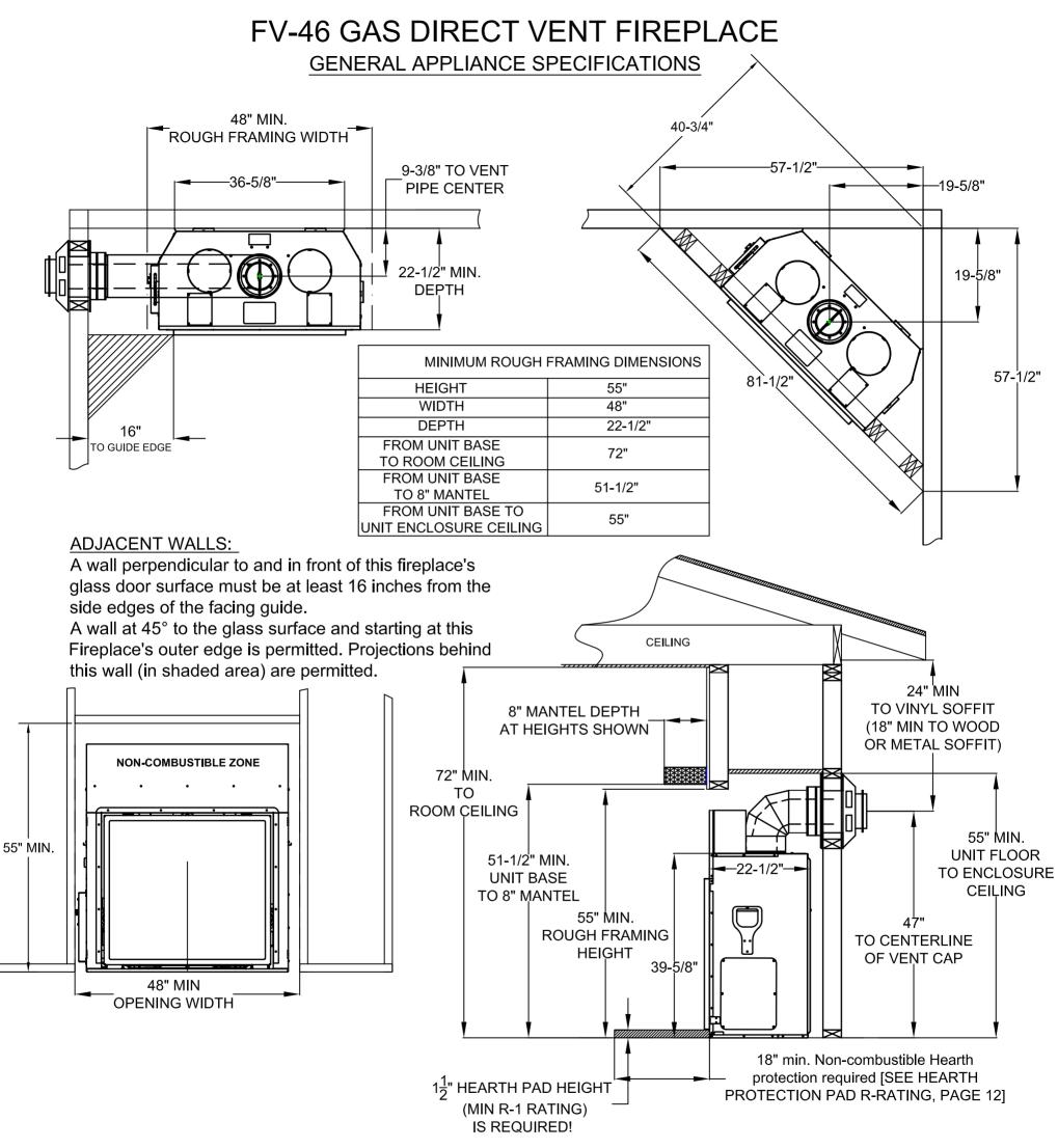
NOTE: For every 1" this fireplace is raised off the floor, the non-combustible hearth protection pad may be reduced by 2". If this fireplace is raised off the floor more than 6", No hearth protection pad is required.
